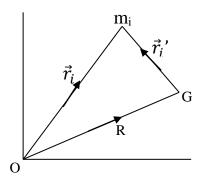
The first term in the R.H.S is the angular momentum of the system about the center of mass G, which is known as the angular momentum of the motion about the center of mass. The second term in the R.H.S is the angular momentum of the single mass m concentrated at the center of mass.
